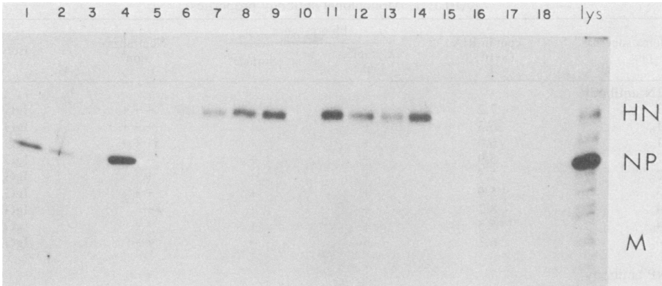
FIG. 1. Immunoprecipitation of NDV proteins by hybridoma supernatants. [ ^{35} S]methionine-labeled, infected CHO cell lysates were subjected to immunoprecipitation with hybridoma supernatants sampled 3 days after feeding. The immune complexes were collected on rabbit anti-mouse immunoglobulin beads (Bio-Rad Laboratories, Richmond, Calif.), electrophoresed, and autoradiographed as described in the text. Supernatants were sampled from hybridomas, and their immunoprecipitates were electrophoresed in lanes numbered as follows: NP1 (lane 1); NP3 (lane 2); NP4 (lane 3); NP2 (lane 4); IgM1 (lane 5); HN _{2a} (lane 6); HN _{1b} (lane 7); HN _{1c} (lane 8); HN _{4a} (lane 9); HN _{4b} (lane 10); HN _{2b} (lane 11); HN _{4c} (lane 12); HN _{3a} (lane 13); HN _{1b} (lane 14); IgM2 (lane 15); IgM3 (lane 16); IgM4 (lane 17); IgM5 (lane 18); cell lysate (lys).
