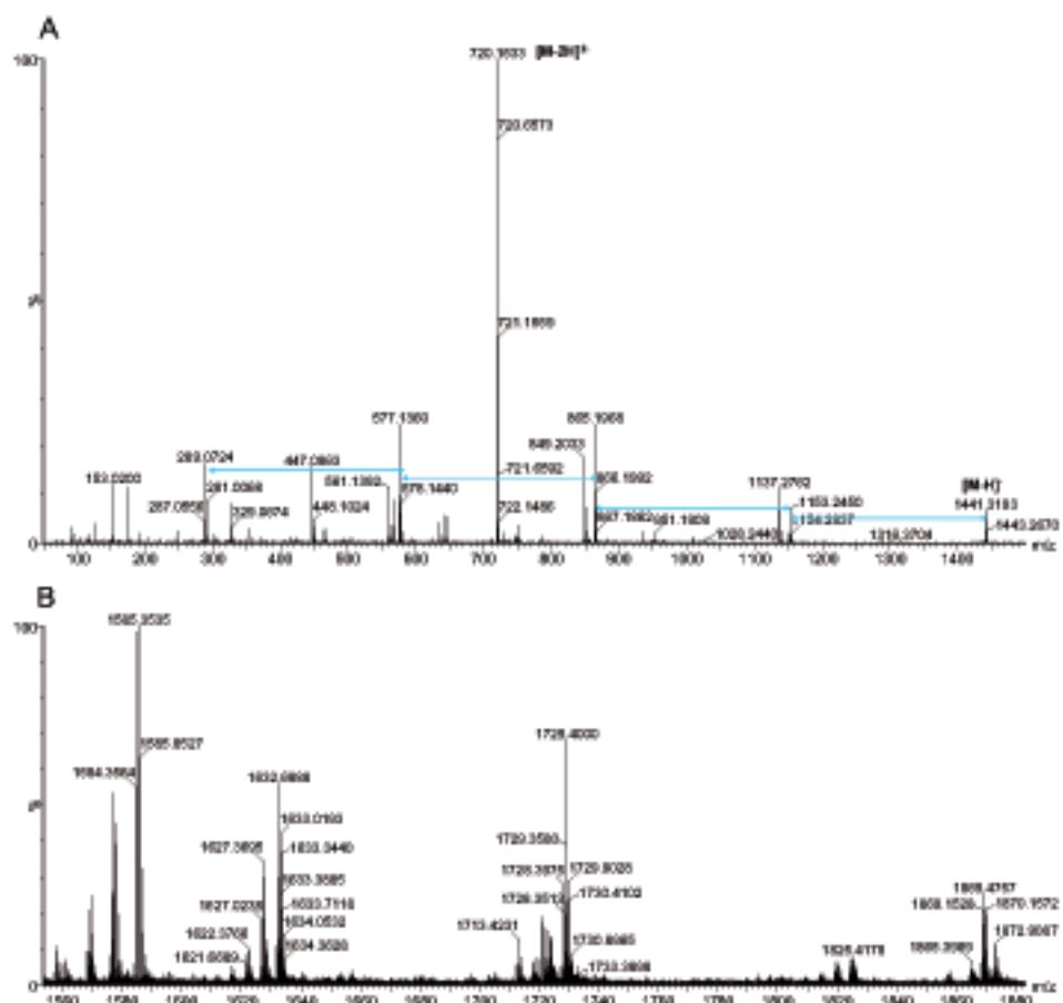
**Figure S2. Procyanidin pentamer MS spectrum.** The single charged ( $m/z$  1441) and double charged ( $m/z$  720) molecular ions are marked on the spectrum. The blue arrows show the fragmentation of catechin units, 288 amu each (A). Tentative procyanidin oligomers larger than ten units (B).
