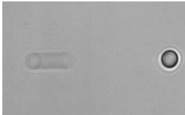
**Movie S1.** Rapid periodic stretching of a lambda phage DNA molecule between two optically trapped beads, as used for cleavage detection of DNA in nonstretched configurations..
