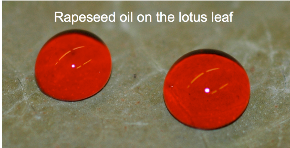
Figure S12. Droplets of rapeseed oil ( \gamma_v = 35.7 mN/m, \eta = 70 mPa.s, \theta = 86^\circ , \theta^* = 141^\circ ) on a lotus leaf dip-coated in a solution of fluorodecyl POSS.
