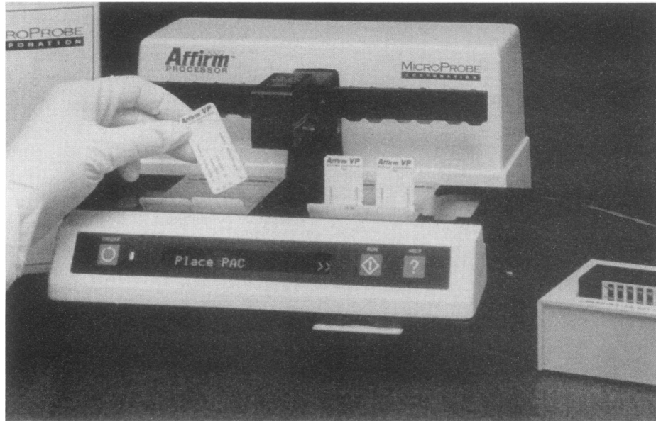
FIG. 1. Microbial nucleic acids were extracted and placed into the first well of the seven-well caddy of the Affirm processor. The reagent cards are moved automatically through the other wells for hybridization and color development, and the assay is completed in 30 min.
