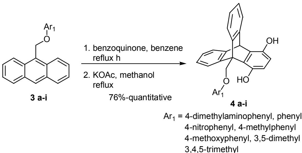
**General Synthetic Procedure for 9-(4-Substituted phenoxy)methyl-1,4-Dihydroxyl triptycene (4).**<sup>3,4</sup> The 9-(aryloxymethyl)anthracene (**3**) (0.8 mmol) and p-benzoquinone (0.26 g, 2.4 mmol) in 4 ml of benzene were refluxed under a nitrogen atmosphere for 1-2 days. After cooling, the solvent was removed under reduced pressure and the formed Diels-Alder adduct was used directly for the aromatization without purification.
