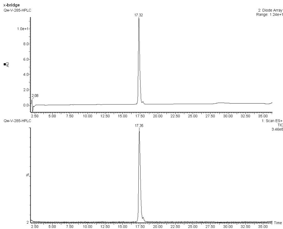
**Figure 58:** UV and MS traces from LC-MS analysis of compound **19**: gradient 20-50% CH<sub>3</sub>CN/H<sub>2</sub>O over 30 min at a flow rate of 0.2 mL/min, X-bridge column
