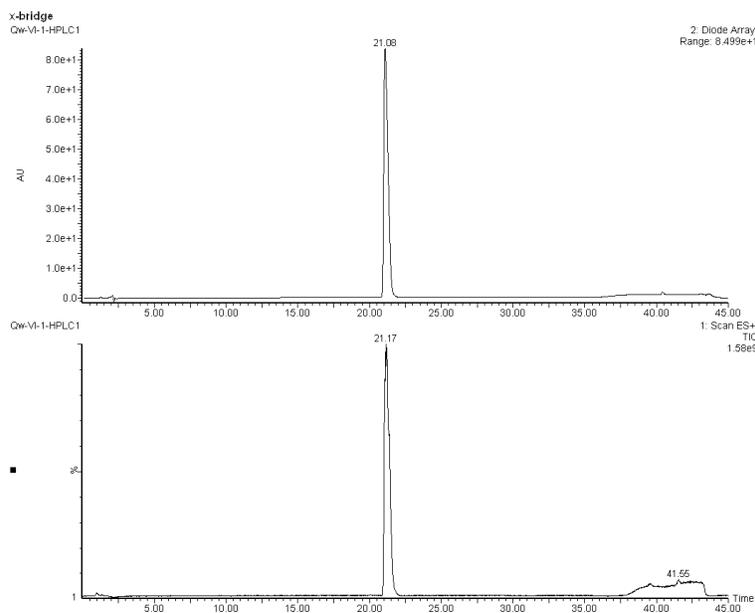
**Figure 64:** UV and MS traces from LC-MS analysis of compound **21**: gradient 20-50%  $CH_3CN/H_2O$  over 30 min at a flow rate of 0.2 mL/min, X-bridge column
