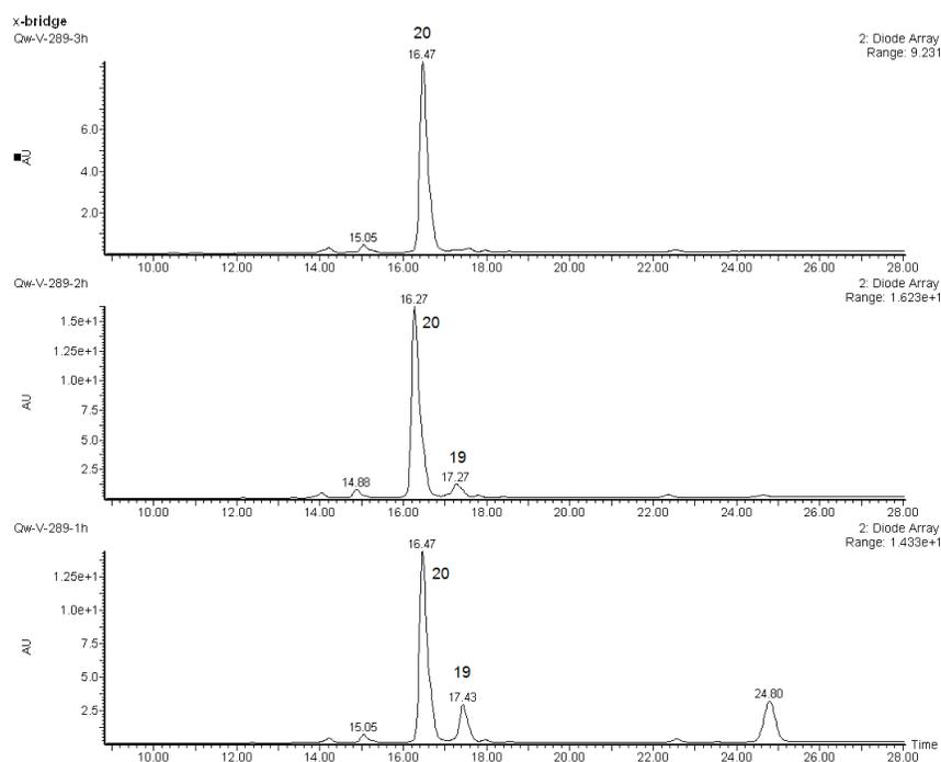
**Figure 60:** UV traces from LC-MS analysis of desulfurization: gradient 20-50%  $\text{CH}_3\text{CN}/\text{H}_2\text{O}$  over 30 min at a flow rate of 0.2 mL/min, X-bridge column
