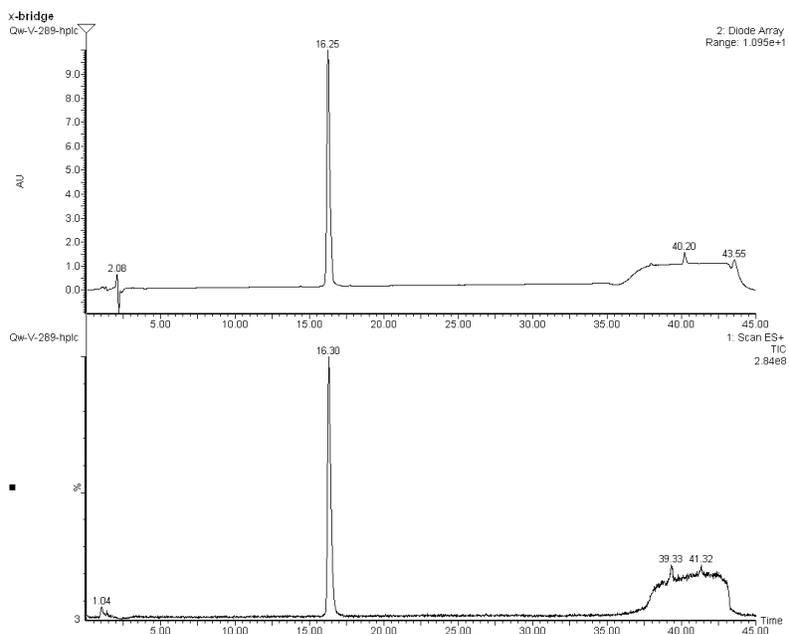
**Figure 62:** UV and MS traces from LC-MS analysis of compound 20: gradient 20-50% CH<sub>3</sub>CN/H<sub>2</sub>O over 30 min at a flow rate of 0.2 mL/min, X-bridge column
