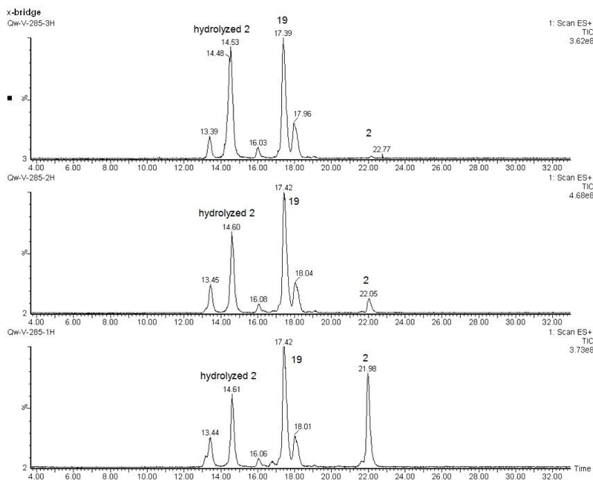
**Figure 57:** MS traces from LC-MS analysis of the ligation: gradient 20-50% CH<sub>3</sub>CN/H<sub>2</sub>O over 30 min at a flow rate of 0.2 mL/min, X-bridge column
