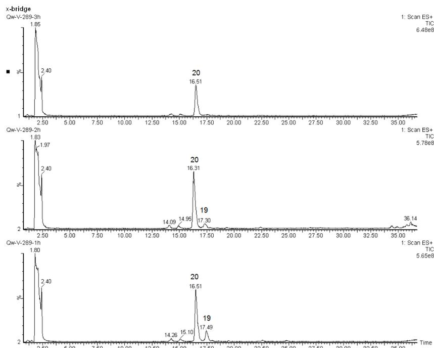
**Figure 61:** MS traces from LC-MS analysis of desulfurization: gradient 20-50% CH<sub>3</sub>CN/H<sub>2</sub>O over 30 min at a flow rate of 0.2 mL/min, X-bridge column
