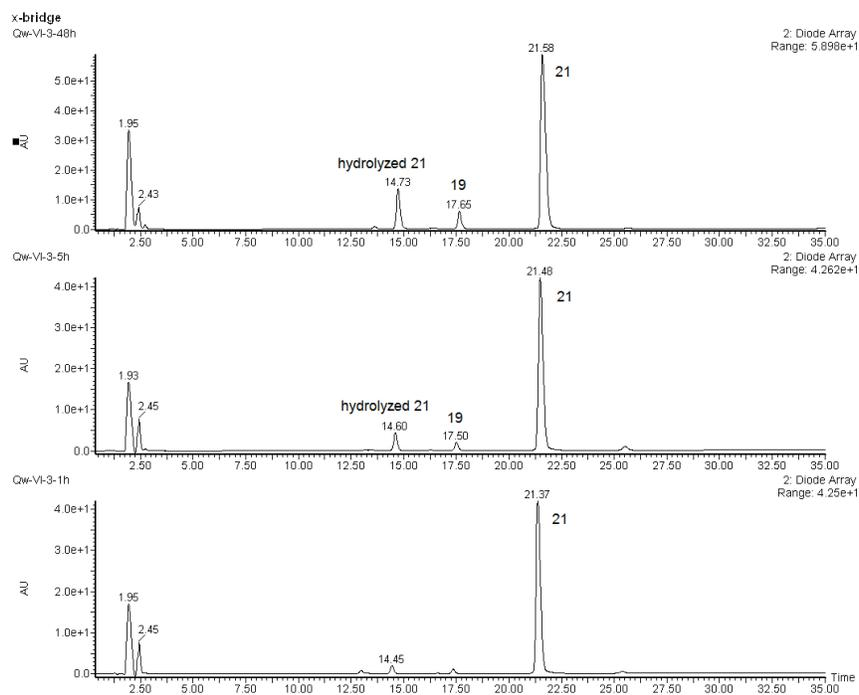
**Figure 65:** UV traces from LC-MS analysis of Pen-ligation: gradient 20-50% CH<sub>3</sub>CN/H<sub>2</sub>O over 30 min at a flow rate of 0.2 mL/min, X-bridge column
