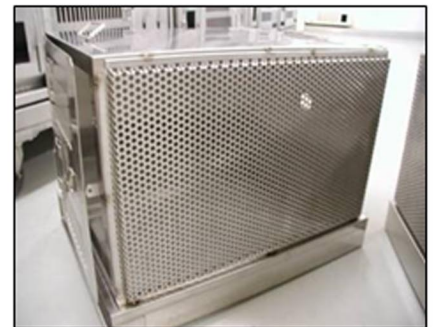
Fig. S3. Transmission model: Respiratory droplet transmission and direct contact transmission. For the respiratory droplet transmission experiments ( Left ), ferrets were housed in adjacent transmission cages, each modified so that a side wall was replaced with a stainless-steel, perforated wall with holes 1–5 mm in diameter and spaced 3 mm apart to facilitate the transfer of respiratory droplets through the air while preventing direct contact between ferrets and indirect contact with the bedding and food of neighboring ferrets. The use of the term “respiratory droplet transmission” throughout this article refers to transmission in the absence of direct or indirect contact and does not imply an understanding of the droplet size involved in virus spread between ferrets. A total of 6 ferrets were used for each respiratory droplet transmission experiment. Three ferrets were inoculated with virus and each was placed in a separate cage. Twenty-four hours later (day 1 p.i. for the inoculated ferrets and day 0 p.c. for the contact ferrets), 3 naive ferrets were each placed in a cage adjacent to an inoculated ferret. To prevent inadvertent physical transmission of virus by the investigators, the contact ferrets were always handled first, and all items that came into contact with the ferrets or their bedding were decontaminated between each ferret. For direct contact transmission experiments, 3 ferrets were each placed in an unmodified cage with solid walls and inoculated with virus. Twenty-four hours later, a naive ferret was placed in the same cage with each inoculated ferret.
