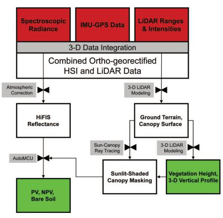
Fig. S2. The processing stream for in-flight and postflight integration of airborne imaging spectrometry and LiDAR observations, shade masking, and fractional canopy cover mapping. Raw data inputs from the CAO are shown in red; computer algorithms are depicted in gray. Final outputs are shown in green.
