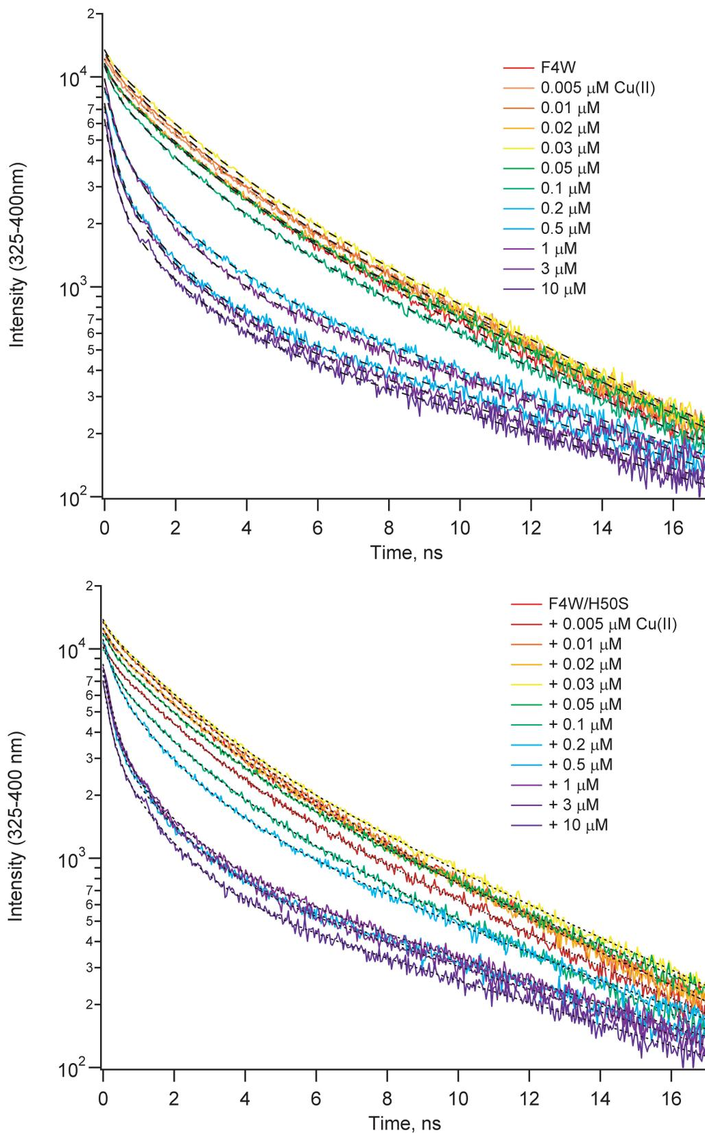
Figure 4S. Trp4 fluorescence decay kinetics as a function of Cu(II) added. F4W (top) and F4W/H50S (bottom); [protein]= 100 nM in 20 mM MOPS, 100 mM NaCl, pH 7. Dotted lines are NNLS fits.
