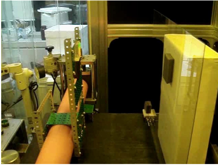
Movie S1. This movie clip shows the transport of a large-area LCD glass by using a dry-adhesive patch with slanted nanohairs. The glass used in the movie is 0.9 mm in thickness, 47.5 \times 37.5 cm 2 in area, and 470 g in weight.
