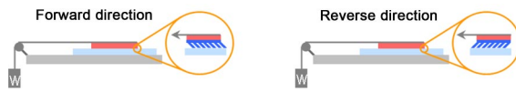
Fig. S2. Schematic illustrations of macroscopic, shear adhesion test, with the definitions of “forward direction” and “reverse direction” with respect to the angle of slanted hairs.
