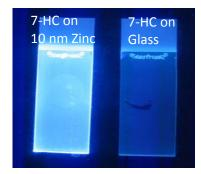
Real-color photographs of 7-HC emission from 10 nm zinc (left) and glass (right) substrates taken through an emission filter.
