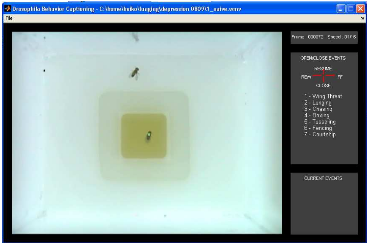
Figure 4: Labeling software for annotating movie sequences by hand and producing ground truth. The user can load and play a movie at different speeds, stop at any frame, go back and forward frame by frame, label start- and end-frame of an event, and chose the event type from the list on the right-hand side.
