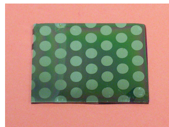
Figure S3 Picture of capacitors for “k” measurements formed with mesoporous silica film on Au-coated Si substrate and 2.5 mm Al electrodes on top
