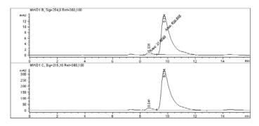
HPLC chromatogram of **20** (Chiralpak AD, 0.8 mL/min, 98:2 hexanes/ethanol, 20 bar, retention rimes: 8.63 (4.1%) and 9.73 (95.8%)).
