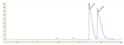
GC chromatogram of rac-19 (HP 6890 GC system with Chiraldex BDM column, 1.5 mL/min, 100°C; retention times: 12.88 min (50.0%) and 13.68 min (50.0%)).
