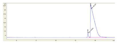
GC chromatogram of **19** (HP 6890 GC system with Chiraldex BDM column, 1.5 mL/min, 100°C; retention times: 13.26 min (2.9%) and 13.55 min (97.0%)).
