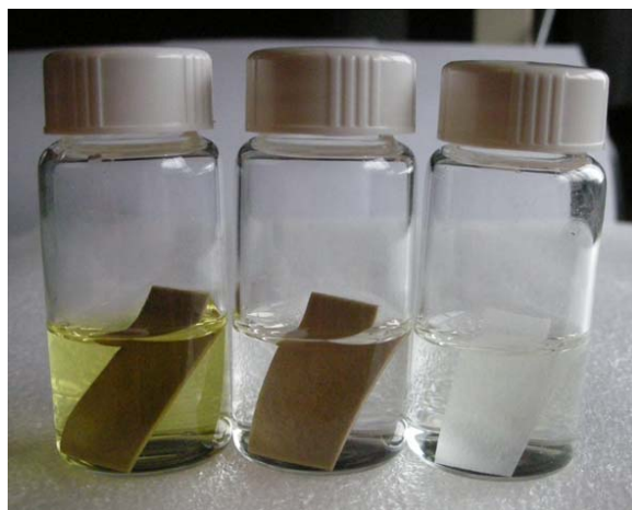
Figure S1. Photographs of trypsin immobilized polydopamine-coated cellulose paper after incubation in the presence of BAPNA for 120 min. The development of yellow color indicates the presence of active trypsin. Samples shown in the photo are trypsin/polydopamine/cellulose (left), polydopamine/cellulose (middle) and unmodified cellulose incubated in trypsin solution and then rinsed with water before the enzymatic reaction (right).
