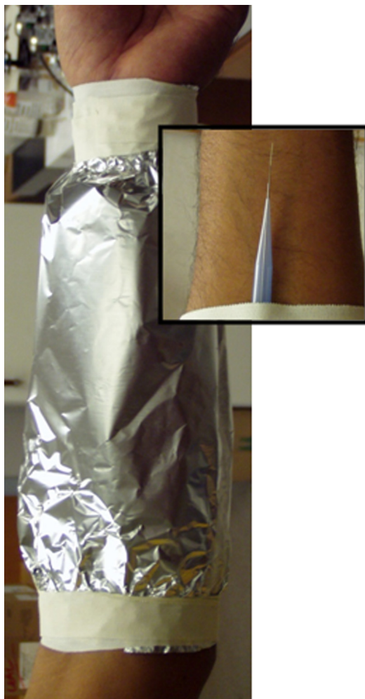
Fig. S1. Set-up for SPME collection of volatiles from the forearm of a human volunteer. A SPME gray fiber ( Inset ) is held by a 1 mL pipette tip and cloth tape to avoid direct contact with the skin. Forearm is enclosed in an aluminum foil with both ends loosely tied with cloth tape.
