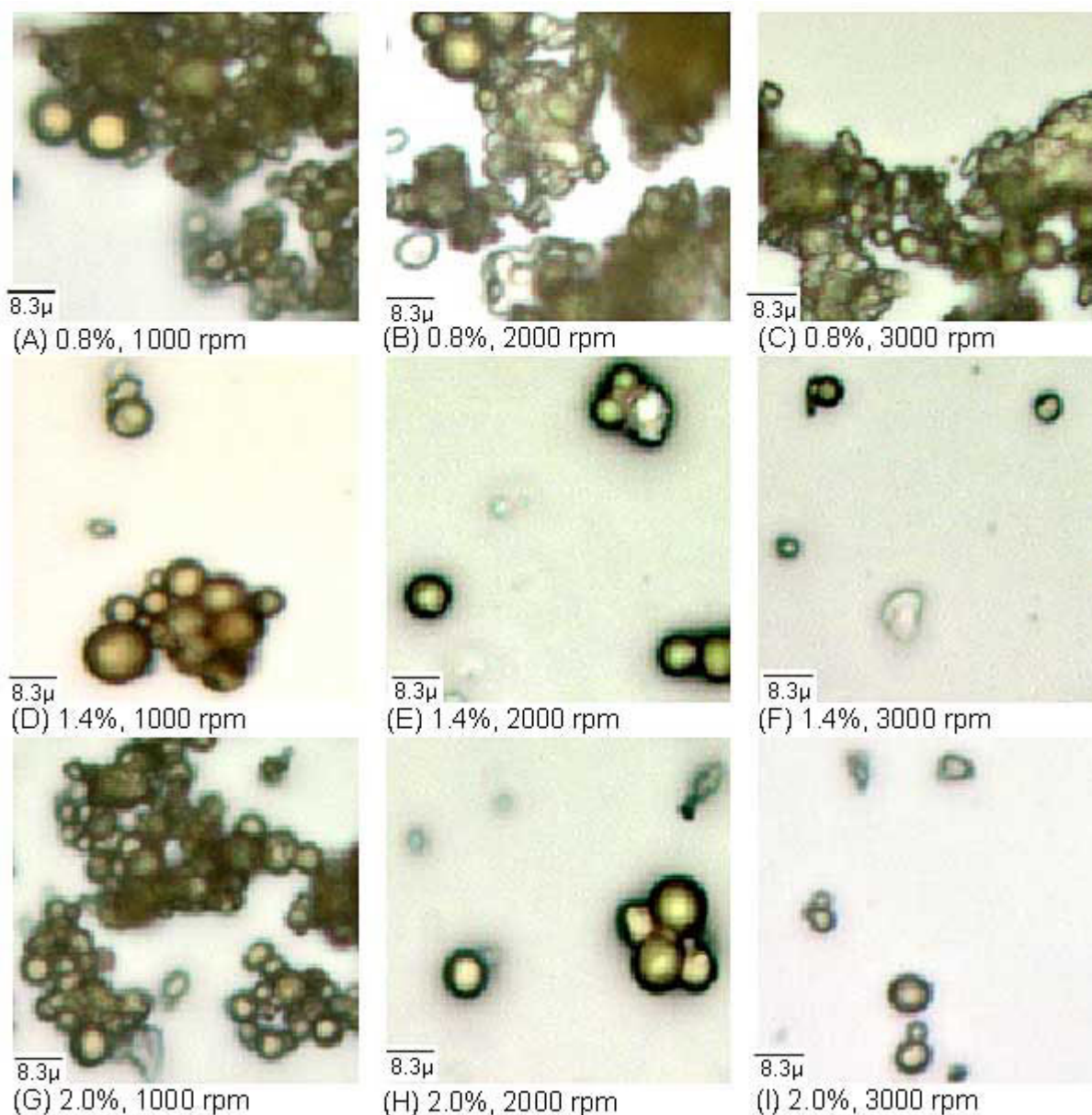
Figure 1. Photomicrographs of unloaded chitosan microspheres prepared using chitosan solution of different concentration (mg/mL chitosan solution) at different stirring speed (rpm) (original magnification \times 1200 ).
