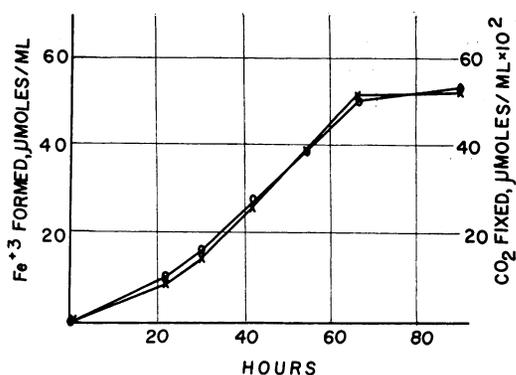
Figure 2. Correlation of ferrous ion oxidation and carbon dioxide fixation during growth of the iron-oxidizing bacterium. Medium M (125 ml) was inoculated with 15 ml of a stationary culture.  $\text{NaHC}^{14}\text{O}_3$  was added. Incubation was at 30 C. X =  $\mu\text{moles ferric ion formed per ml}$ ; O =  $\mu\text{moles CO}_2$  fixed per ml  $\times 10^2$ .
