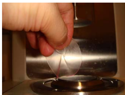
Figure S3. Picture of the hydrogel containing 20% macromonomer 1 and 20% macromonomer 3b (1:1) in 100 mM \text{NH}_4\text{HCO}_3 , pH 8.3 after oscillatory rheology (rheology method 1).
