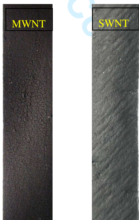
Figure S1. Optical photographs of the MWNT and SWNT coated paper electrodes.
