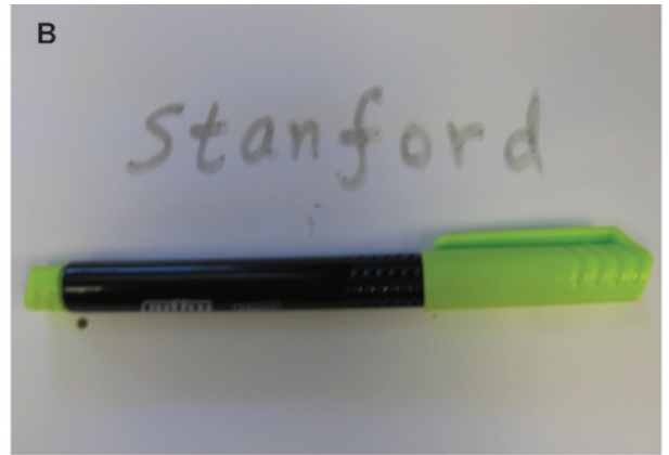
Fig. S3. Properties of CNT films. (A) The global and local sheet resistances for PET and paper before and after the surfactant washing process. The error ranges of all of the bars presented here and in Fig. 2A are \pm 10\% . (B) The writing of CNT ink by using a highlighter pen.
