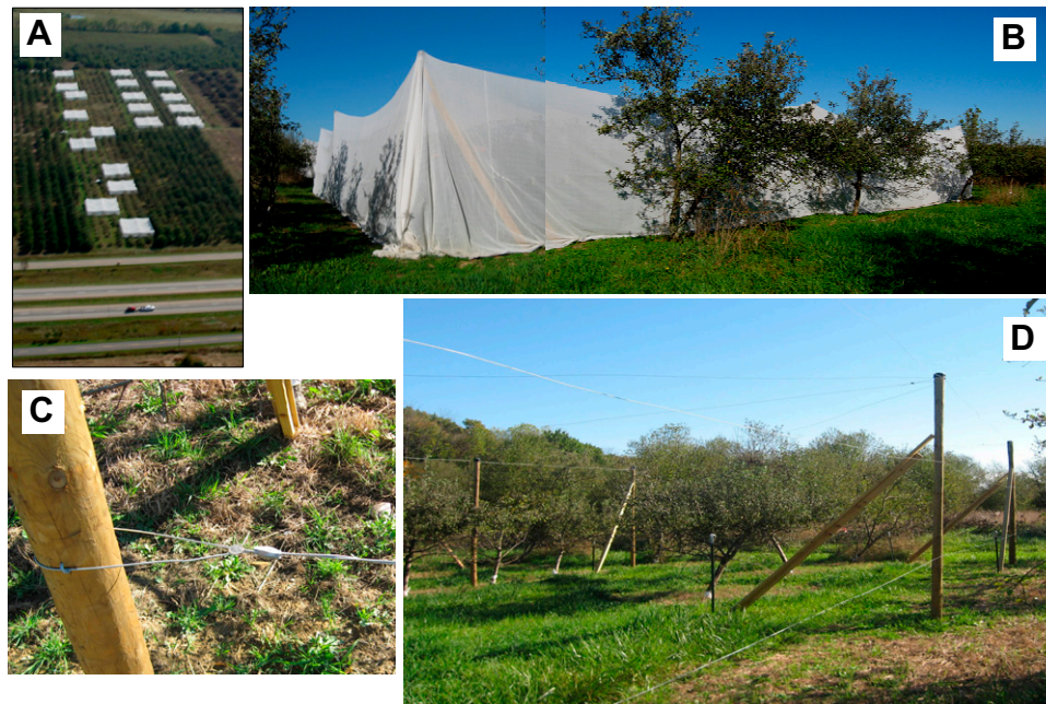
Fig. S1. (A) Aerial photograph of the 20 large field cages; note size of automobile towing trailer on interstate highway. (B) Individual cage measuring 19 \times 19 \times 3.5 m and covering 12 apple trees. (C) Gripper apparatus for tightening trellis wires. (D) Elements of cage superstructure: posts, braces, trellis wire. (E) Shade cloth used as netting for a single cage laid out for preinstallation folding. (F) Net installation. (G) Half of the interior of one cage. (H) Monitoring trap showing high catch of codling moth males on the sticky liner covering trap bottom. (I) J.R.M. checking trap. (J) Codling moth male. (K) Cages used to deploy individual females in traps.
