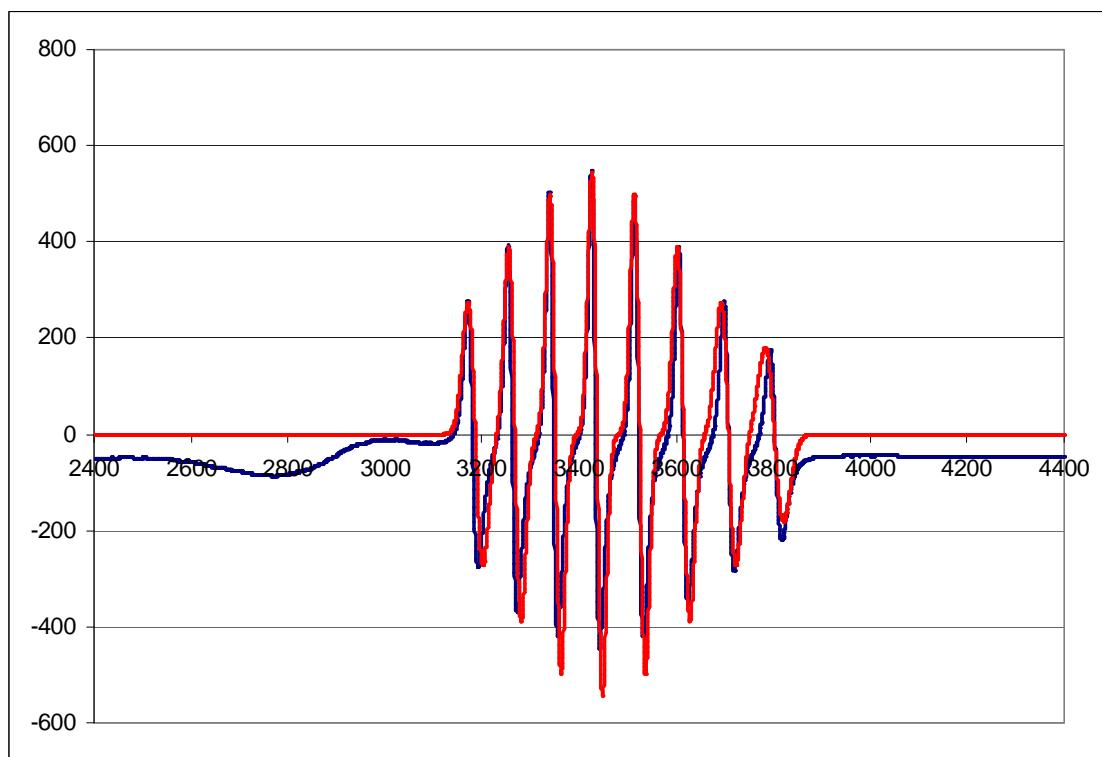
(f)  $V^{IV}$ O-cyclam chloride, **2** in methanol at 77 K
