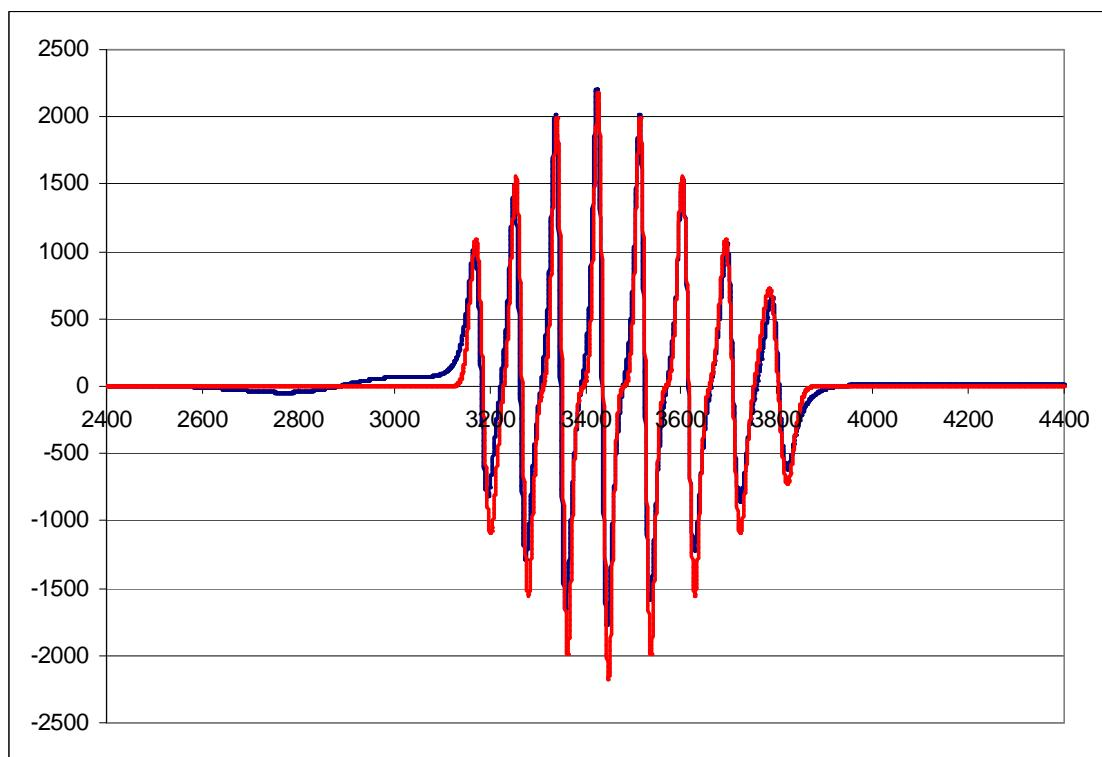
(c) V<sup>IV</sup>O-cyclam sulfate, **1** in methanol at 77 K
