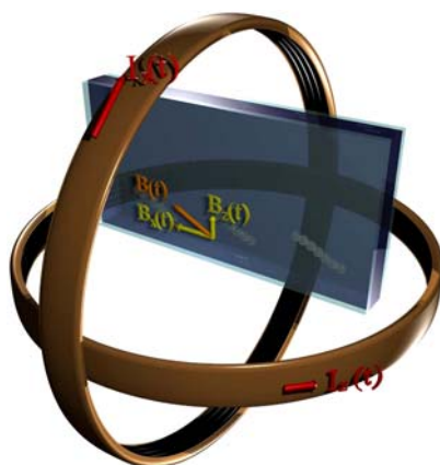
Fig. S1. A figure demonstrating the experimental setup used to probe the behavior of superparamagnetic colloids. Phase-shifted sinusoidal currents I_x and I_z impart a rotating magnetic field at the center of the coils. Not shown is a viewing window through the coils where they intersect to allow for sideways viewing of the rotors.
