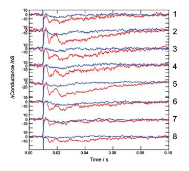
**Fig. S3.** Synaptic blocker test for 2D Si NWFET array. The conductance change in devices 1–8 (as labeled in Fig. 5*A*) were recorded when stimulating with a 200 µs, 400 µA current pulse (*Red Traces*). CNQX and APV were then applied and devices were recorded with the same parameters (*Blue Traces*). The results show that recorded signals from all devices were blocked by CNQX and APV.
