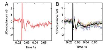
**Fig. S2.** Comparison between single raw traces and averaged data. (*A*) A representative raw single data trace recorded from a NWFET. (*B*) Six raw traces (*Dashed Color Lines*) recorded from NWFET overlaid with the averaged of the six (*Solid Black Line*). Averaged results were used to accurately identify the peak position and peak width for comparison across different devices and samples.
