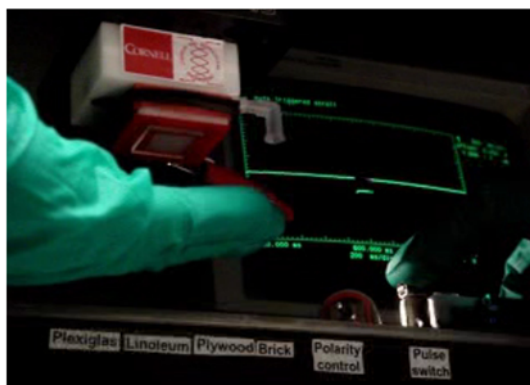
Movie S1. Reversible wet adhesion: Demonstration of concept in substrate-pendant mode. First substrate (Plexiglas) is 2 \text{ cm} \times 2 \text{ cm} . The voltage pulse to attach is displayed on the oscilloscope (grab/release pulses are \pm 15 \text{ V} ). Note footprints left on Plexiglas substrate after release. Device is MS (machine shop), N = 10 \times 10 , \epsilon = 440 \mu\text{m} .
