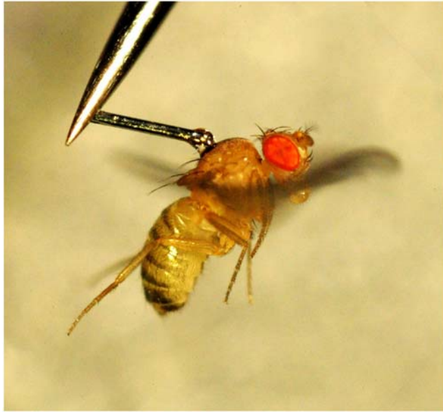
Fig. 51. A common fruit fly ( D. melanogaster ) with ferromagnetic pin glued to the dorsal surface of its thorax is suspended by a magnetized sewing needle. The pin is 1.5 mm long. In free flight, the insect is perturbed by application of a magnetic field that induces a torque on the pin.
