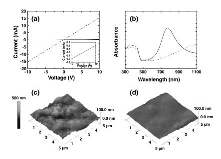
Fig. S6. (A) I-V characteristics and (B) UV-vis-NIR spectra of untreated (solid lines) and DCA-treated (dashed lines) PANI-PSS films. Inset of (A): magnified plot of the I-V characteristics of untreated PANI-PSS film. AFM images of (C) untreated (rms roughness of  $\approx$ 13.7 nm) and (D) DCA-treated (rms roughness of  $\approx$ 2.9 nm) PANI-PSS films.
