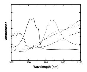
Fig. S10. UV-vis-NIR spectra of P3HT (solid line), untreated (dashed line) and DCA-treated (dash-dotted line) PANI-PAAMPSA, and untreated (dotted line) and DCA-treated (dash-double-dotted line) PEDOT-PSS.
