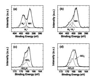
Fig. S5. XPS nitrogen spectra of (A) untreated and (B) DCA-treated PANI-PAAMPSA, and sulfur spectra of (C) untreated and (D) DCA-treated PANI-PAAMPSA, respectively. The deconvoluated peaks are shown as dotted lines.
