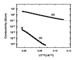
Fig. 52. Temperature-dependent conductivities of (A) untreated PANI-PAAMPSA and (B) DCA-treated PANI-PAAMPSA films collected by two-point probe and four-point probe measurement, respectively. The dashed lines represent fits to data with Eq. 51.
