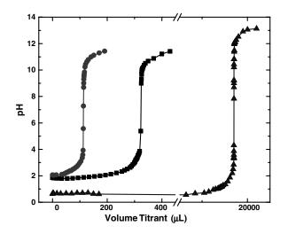
Fig. S1. Titration curves of (A) DCA (pK<sub>a</sub>  $\approx$  0.70;  $\blacktriangle$ ), (B) PAAMPSA (pK<sub>a</sub>  $\approx$  2.29;  $\textcircled{\bullet}$ ), and (C) PSS (pK<sub>a</sub>  $\approx$  1.95;  $\blacksquare$ ). Titration was carried out with 0.1 M sodium hydroxide at 70 °C.
