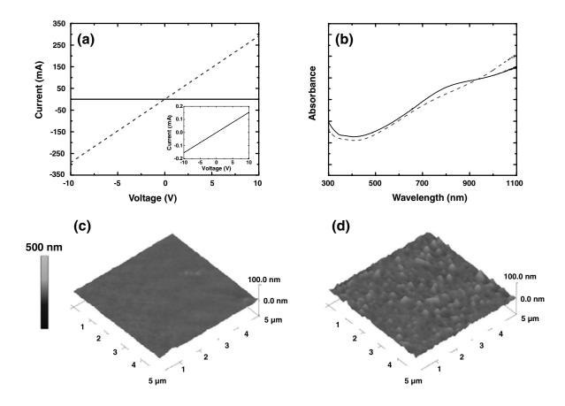
**Fig. S8.** (A) *I–V* characteristics and (B) UV-vis-NIR spectra of untreated (solid lines) and DCA-treated (dashed lines) PEDOT-PSS films. Inset of (A): magnified plot of the *I–V* characteristics of the untreated PEDOT-PSS film. AFM images of (C) untreated (rms roughness of  $\approx$ 0.9 nm) and (D) DCA-treated (rms roughness of  $\approx$ 2.6 nm) PEDOT-PSS films.
