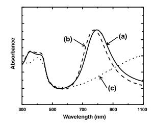
Fig. S4. UV-vis-NIR spectra of (A) HCI-treated, (B) untreated, and (C) DCA-treated PANI-PAAMPSA.
