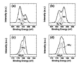
Fig. S7. XPS nitrogen spectra of (A) untreated and (B) DCA-treated PANI-PSS, and sulfur spectra of (C) untreated and (D) DCA-treated PANI-PSS, respectively. Deconvoluted peaks are shown as dotted lines.
