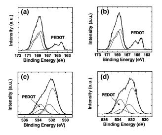
Fig. S9. XPS sulfur spectra of (A) untreated and (B) DCA-treated PEDOT-PSS, and oxygen spectra of (C) untreated and (D) DCA-treated PEDOT-PSS, respectively. Deconvoluted peaks plotted with dotted lines.
