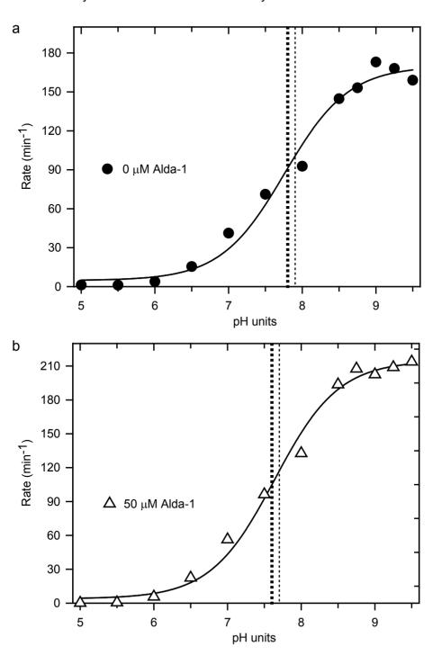
**Supplementary Figure 1** Dependence of ALDH2-catalyzed hydrolysis of para-nitrophenylacetate on pH. The rate of nitrophenol formation by ALDH2-catalyzed hydrolysis of para-nitrophenylacetate was monitored as a function of pH in the absence (a) and presence (b) of 50 uM Alda-1. In each panel, the apparent pKa values for ester hydrolysis are indicated by the dashed vertical lines (pKa = 7.8 in the absence of Alda-1 and pKa = 7.6 in the presence of Alda-1).
