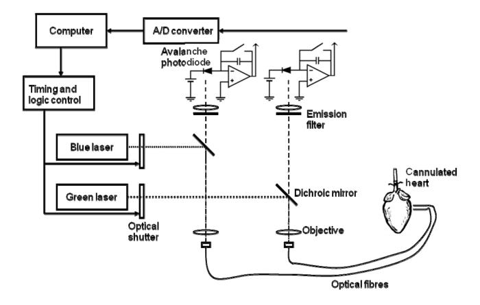
**Supplementary figure 1.** Scheme of the experimental setup for detecting whole heart fluorescent signals. A solid state blue laser (473 nm) was used to excite mag-fluo-4 and a solid state green laser (532 nm) was used to excite rhod-2, X-rhod-5F, and Di-8-ANEPPS. Both lasers were time-multiplexed by two ferroelectric modulators (optical shutters). The fluorescence
