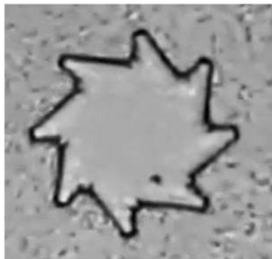
Movie S2. A nanofabricated asymmetric gear (48- \mu\text{m} external diameter, 10- \mu\text{m} thickness) rotates clockwise at 1 rpm when immersed in an active bath of motile Escherichia coli cells, visible in the background. The gear is sedimented at a liquid–air interface to reduce friction. The video plays at twice the original frame rate; a moving crop area guarantees an almost stationary center of mass of the gear.
