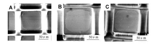
Fig. S2 ESEM images of SU-8 micropallets contact printed with: (A) collagen, (B & C) a 0.1% solution of gelatin after a single stamping (B) and after 4 stampings (C).
