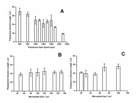
Fig. S1 (A) Plot of polystyrene intrusion length *vs.* polystyrene film spin speed.(B) Plot of polystyrene intrusion length *vs.* micropallet dimension. (C) Plot of polystyrene intrusion length *vs.* gap between the micropallets.
