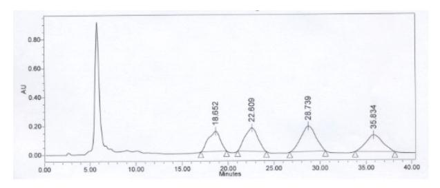
(a) FluoroFlash Column, 100% MeOH, 10 mL/min, 20 mg M-21a,b/a,c in 1 mL MeOH/injection
