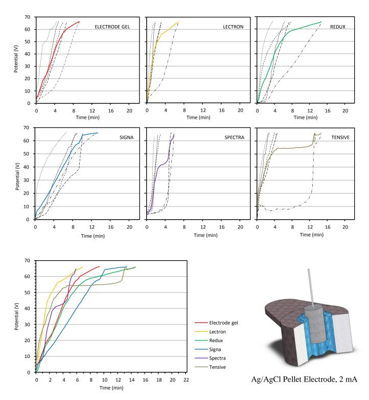
Supplementary Figure 1.B - Current induced polarization of conductive Ag/AgCl pellet electrode, shown as apparent voltage across anode against time. Voltage measured across Ag/AgCl anode is shown against time. 2mA DC current with commercially available gels was passed and change in voltage with time was measured. Black dotted curves shows five repeats while colored line shows average. The lower panel compares average voltage plots of all gels.
