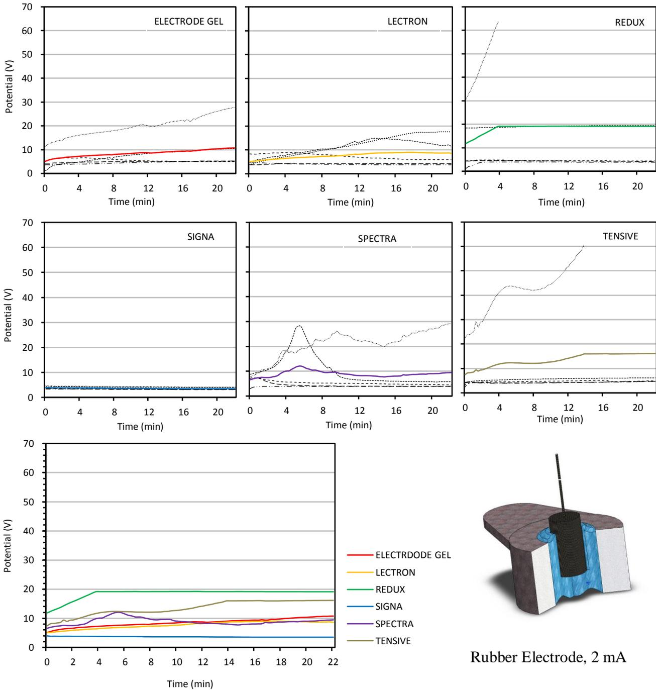
Supplementary Figure 1.C - Current induced polarization of conductive Rubber electrode, shown as apparent voltage across anode against time. Voltage measured across rubber anode is shown against time. 2mA DC current with commercially available gels was passed and change in voltage with time was measured. Black dotted curves shows five repeats while colored line shows the average of five repeats. The lower panel compares average voltage plots of all gels.
