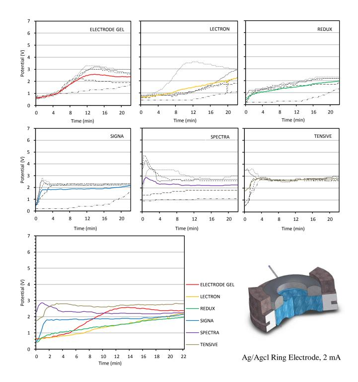
Supplementary Figure 1.D - Current induced polarization of conductive Ag/AgCl Ring electrode, shown as apparent voltage across anode against time. Voltage measured across Ag/AgCl Ring anode is shown against time. 2mA DC current with commercially available gels was passed and change in voltage with time was measured. Black dotted curves shows five repeats while colored line shows the average of five repeats. The lower panel compares average voltage plots of all gels.
