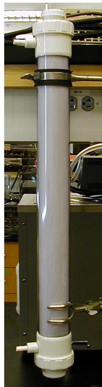
Figure 2. The Kros Flo Plus hollow-fiber unit contained 10 m 2 of polypropylene fibers that were 65 cm long and had a 240 micron OD with 20 micron wall thickness. Buffer flowed through the fibers while a 71 kPa (21" Hg) vacuum was maintained on the shell side.
