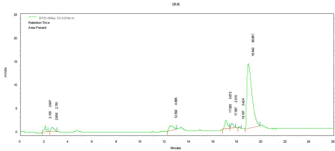
**1,4-disubstituted 1,2,3-triazole member 2{9,9}.** HPLC ( $\text{CH}_3\text{OH} : \text{H}_2\text{O}$ )  $R_T$  14.20 (100%), gradient elution 55% to 95% over 21 min.
