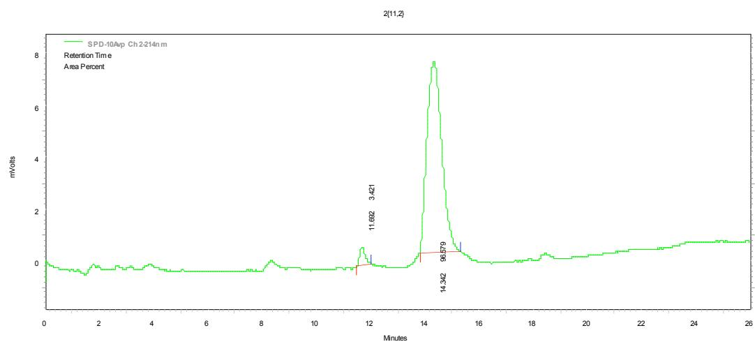
**1,4-disubstituted 1,2,3-triazole member 2{11,3}. HPLC (CH<sub>3</sub>OH : H<sub>2</sub>O) R<sub>T</sub> 14.66 (86%).**
