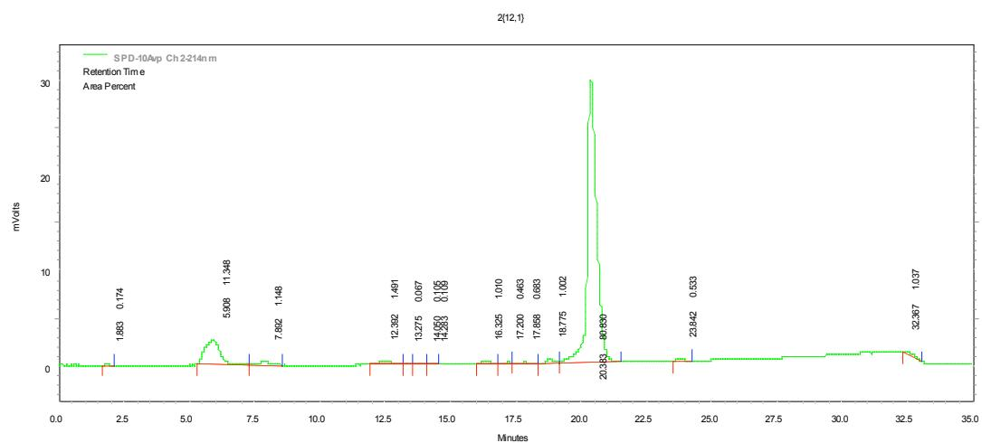
**1,4-disubstituted 1,2,3-triazole member 2{12,2}.** HPLC ( $\text{CH}_3\text{OH} : \text{H}_2\text{O}$ )  $R_T$  20.29 (97%), gradient elution 55% to 95% over 35 min.
