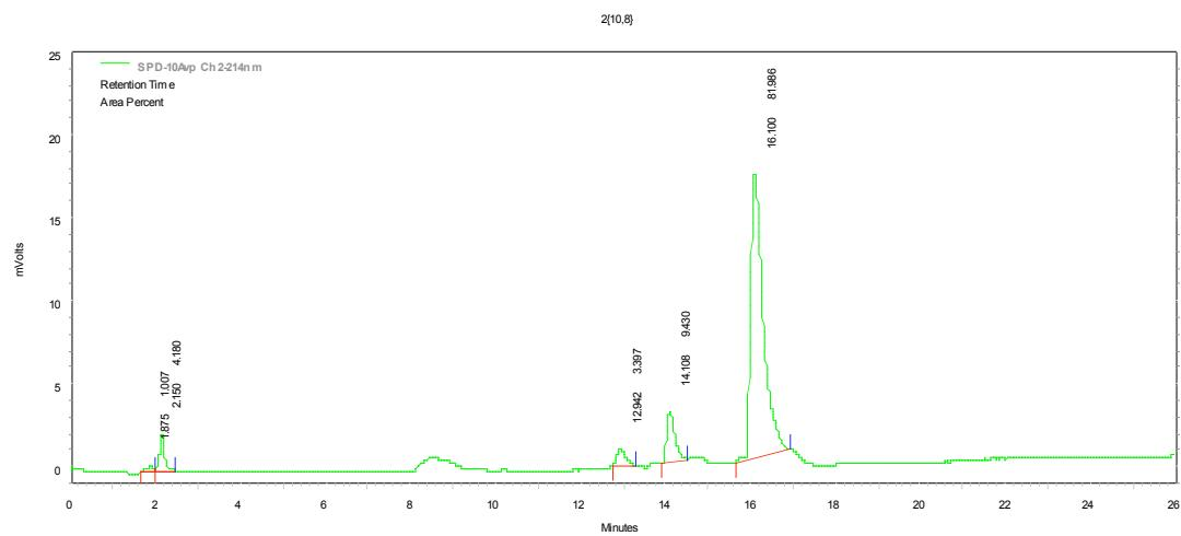
**1,4-disubstituted 1,2,3-triazole member 2{10,9}. HPLC (1% AcOH in  $\text{CH}_3\text{OH} : \text{H}_2\text{O}$ )  $R_T$  3.40 (100%), gradient elution 30% to 90% over 20 min.**
