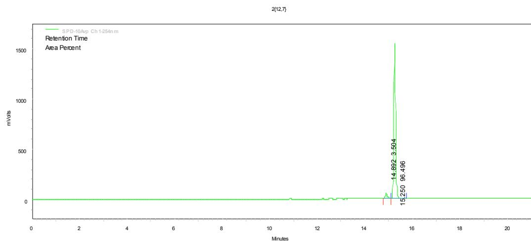
**1,4-disubstituted 1,2,3-triazole member 2{12,8}.** HPLC ( $\text{CH}_3\text{OH} : \text{H}_2\text{O}$ )  $R_T$  13.92 (84%), gradient elution 55% to 95% over 21 min.
