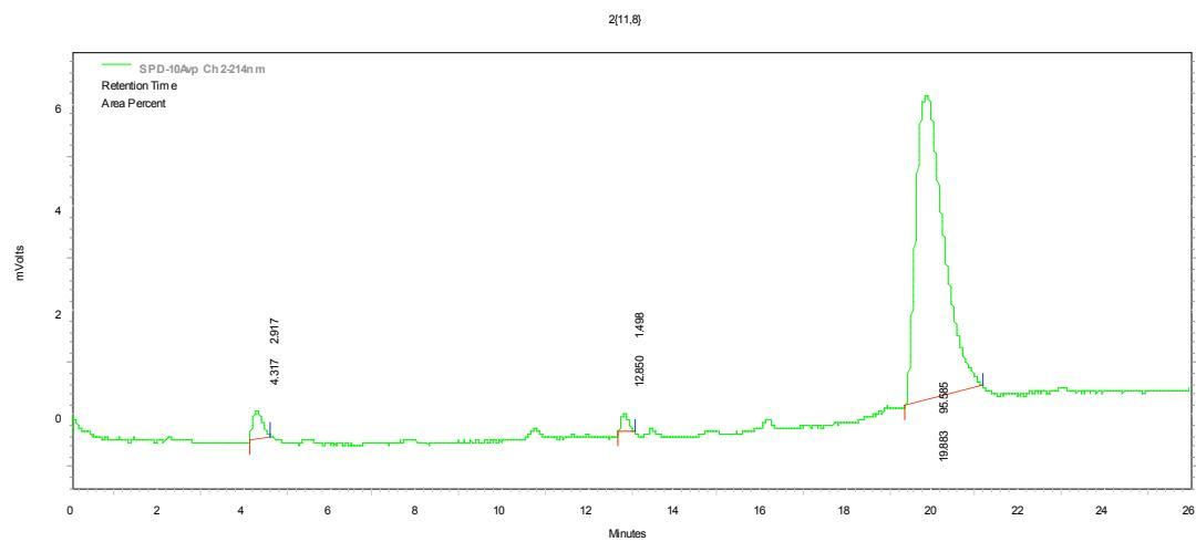
**1,4-disubstituted 1,2,3-triazole member 2{11,9}. HPLC (CH<sub>3</sub>OH : H<sub>2</sub>O) R<sub>T</sub> 17.04 (95%).**
