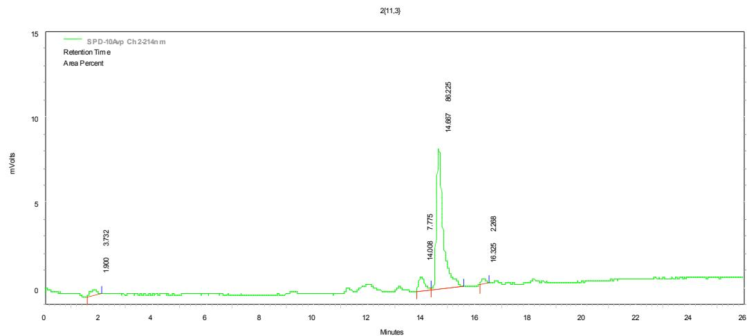
**1,4-disubstituted 1,2,3-triazole member 2{11,4}. HPLC (CH<sub>3</sub>OH : H<sub>2</sub>O) R<sub>T</sub> 16.15 (86%).**
