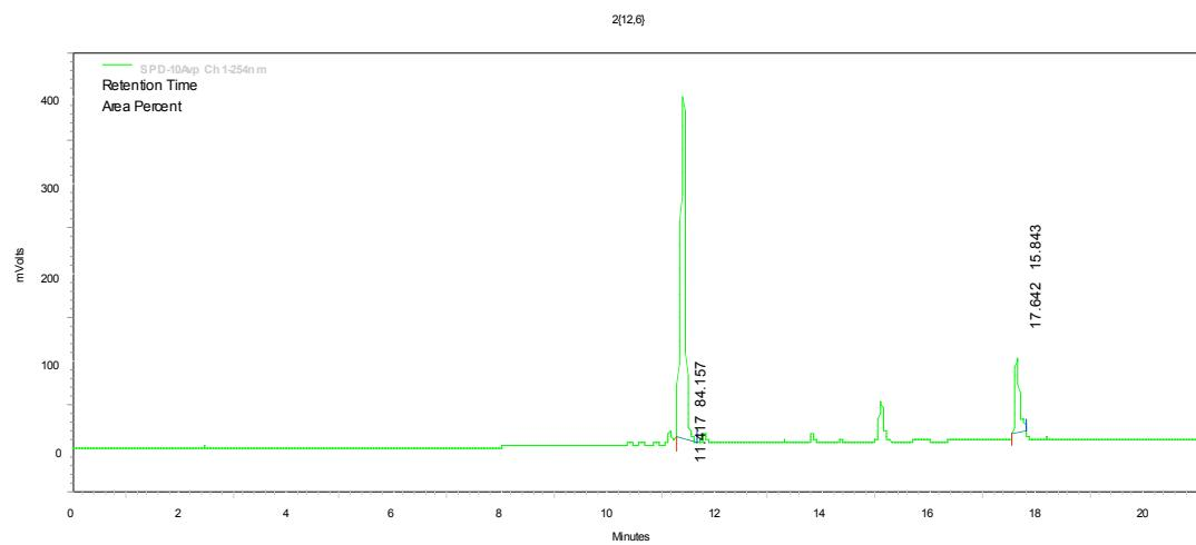
**1,4-disubstituted 1,2,3-triazole member 2{12,7}.** HPLC ( $\text{CH}_3\text{OH} : \text{H}_2\text{O}$ )  $R_T$  15.25 (96%), gradient elution 55% to 95% over 21 min.
