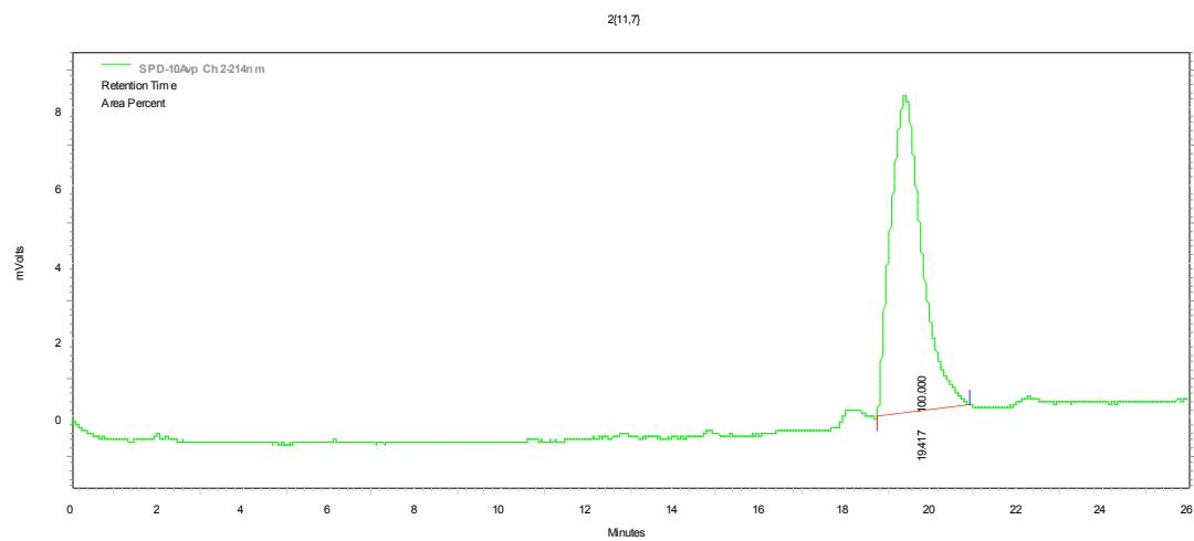
**1,4-disubstituted 1,2,3-triazole member 2{11,8}. HPLC ( $\text{CH}_3\text{OH} : \text{H}_2\text{O}$ )  $R_T$  19.88 (95%).**
