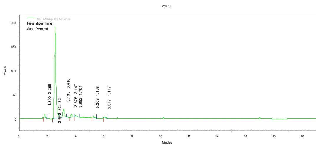
**1,4-disubstituted 1,2,3-triazole member 2{10,2}.** HPLC (1% AcOH in CH<sub>3</sub>OH : H<sub>2</sub>O) R<sub>T</sub> 2.65 (100%), gradient elution 30% to 90% over 21 min.
