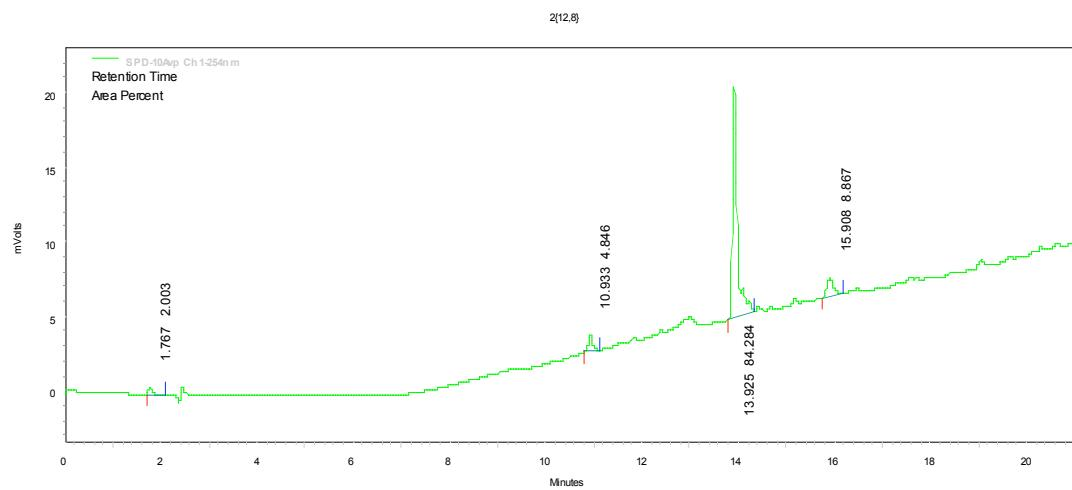
**1,4-disubstituted 1,2,3-triazole member 2{12,9}.** HPLC ( $\text{CH}_3\text{OH} : \text{H}_2\text{O}$ )  $R_T$  10.99 (82%), gradient elution 55% to 95% over 21 min.
