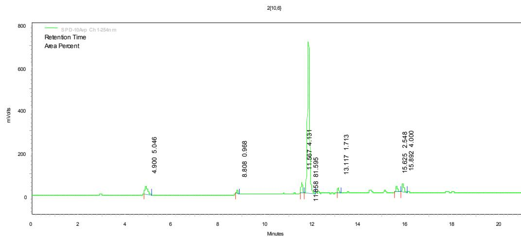
**1,4-disubstituted 1,2,3-triazole member 2{10,7}.** HPLC ( $\text{CH}_3\text{OH} : \text{H}_2\text{O}$ )  $R_T$  16.73 (94%), gradient elution 55% to 95% over 21 min.
