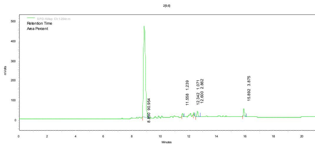
**1,4-disubstituted 1,2,3-triazole member 2{9,7}.** HPLC ( $\text{CH}_3\text{OH} : \text{H}_2\text{O}$ )  $R_T$  12.84 (98%), gradient elution 55% to 95% over 21 min.
