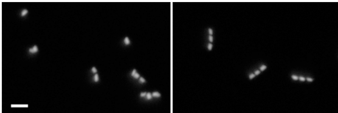
Supporting Figure 1. Reflectance images of Au/Ni striped nanowires coated with 1TEOS:1AcPTES (left) and 3TEOS:1AcPTES (right) with the Ni segment etched, demonstrating that the silica was not thick enough to keep the Au segments together for the 1:1 sample, but did maintain structure when a 3:1 TEOS:AcPTES ratio was used. Scale bar = 2 \mu\text{m} .
