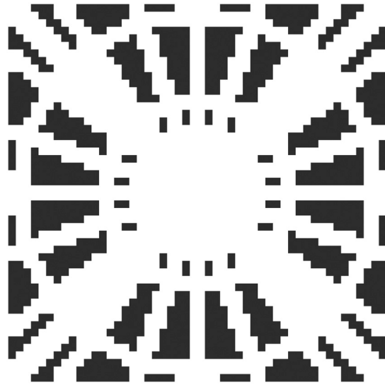
Fig. S2. The real-space pattern of the scattering layer. Black corresponds to high-dielectric regions. White regions are air.
