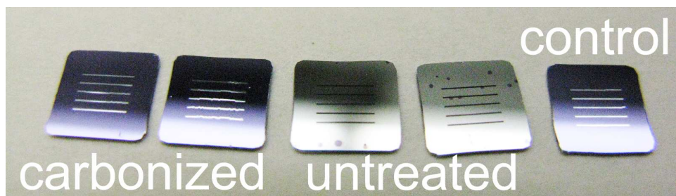
Figure S-4. Carbonized and untreated pnc-Si membranes after 1 hour in %5 KOH at 40°C. The rectangular slits are free-standing pnc-Si. Untreated membranes are discolored indicating the dissolution of the silicon film 3 .
