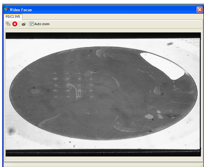
Figure 1S. SPRi image of printed array in PBS buffer. The carbohydrate microarray contained Man3, Man2, Man, Glc, and Gal, printed in quadruplets, fabricated on 90:10 mixed SAM of PFPA-MUTEG/MDEG.
