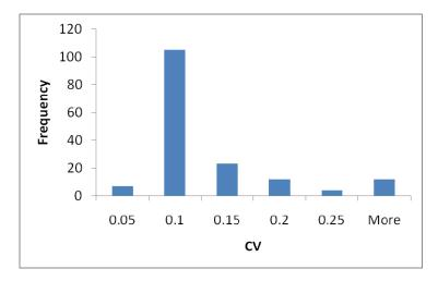
**Experimental variance** (CV) determined based on a study with 45 technical replicates of identical human serum measured on 9 different Biocrates AbsoluteIDQ kit plates (5 replicate samples/kit).
