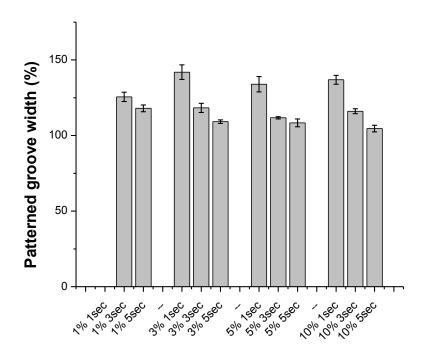
**Figure S1.** Patterned groove width with different UV exposure time and photoinitiator with 1, 3, 5, 10% concentration. Higher initial photoinitiator concentration requires shorter exposure time for patterning. The first condition (PI concentration: 1%, exposure time: 1 sec) was not measurable due to the under-crosslinked structure. Photomask width = 320 μm, spacer thickness = 150 μm (one coverslip) with constant UV intensity (7.5 mW/cm²).
