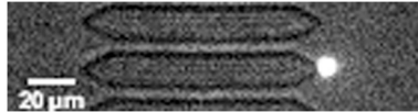
Movie S1. RBCM particles (1% cross-linked) that are 6 \mu\text{m} in diameter deforming in flow to traverse a 3- \mu\text{m} wide restriction in a 3- \mu\text{m} tall poly(dimethyl siloxane) microfluidic channel. Observed restrictions are in the middle of the device, implying that the RBCMs in this movie have traversed approximately 50 such pores immediately prior to imaging without noticeable loss of structure or elasticity. The flow rate was 0.06 \mu\text{L}/\text{min} .
