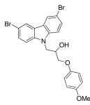
Following Representative Procedure 1, **43** was prepared in 47% yield from dibromocarbazole and (*p*-methoxyphenyl)-glycidyl ether with NaH as the base.
