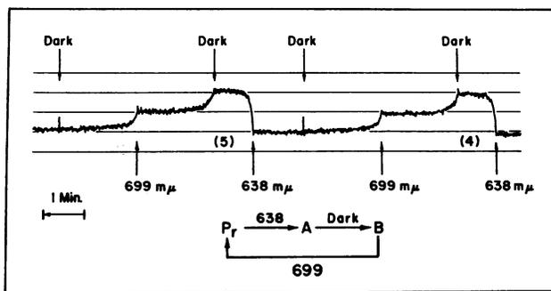
FIG. 2.—Spectrophotometer (Cary 14) tracing of absorption changes at 695 nm of  $P_r$  solution at  $-77^\circ$ ; cycle: 638 nm, dark, 699 nm, dark; time, increasing to left; absorbance scale, 0.005 per vertical division. The fourth and fifth cycles are shown. A,  $R_1$ ; B,  $R_2$ .
