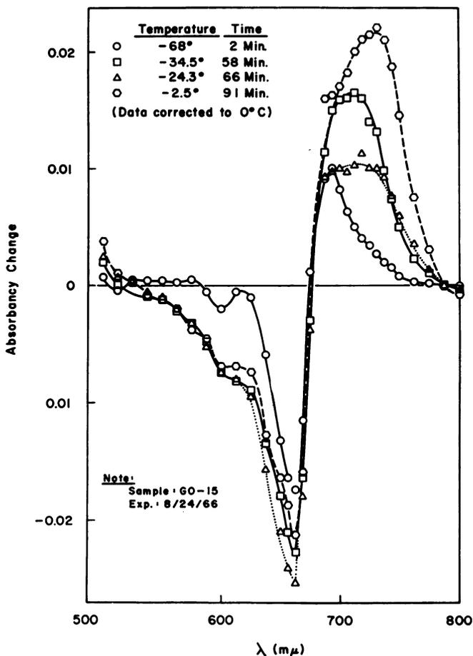
FIG. 3.—Absorption spectral changes in  $P_r$  upon slow warming in dark after irradiation at  $-68^\circ$ . Indicated elapsed time between cessation of illumination and beginning of each (5-min) scan. First intermediate (○) is  $R_2$ . Spectra corrected for volume change with temperature.
