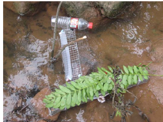
Photo S1: Direct sampler in situ . The direct sampler (A) is deployed in the site of interest in parallel with the mouse bioassay cage (B) seen here with a sun cover.
