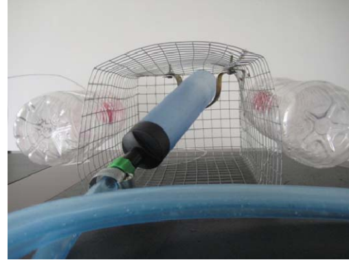
Photo S2: Siphon sampler. Posterior view of siphon sampler including external floats and siphon tubing.
