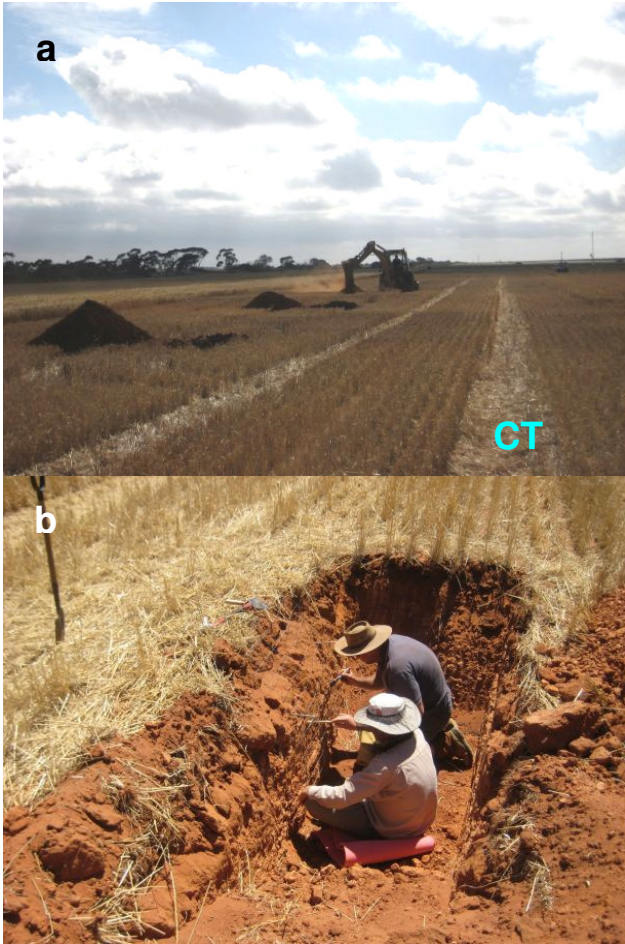
Supplementary Figure S4 | Assessing insect tunnels in plots. (a) Backhoe digging holes in plots; CT = controlled traffic tracks. (b) Counting tunnels in quadrats on wall of hole.
